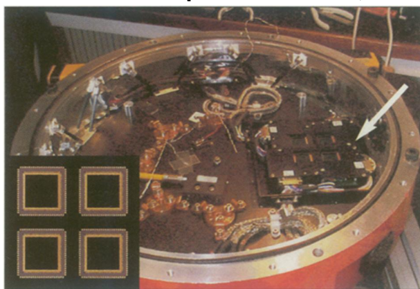
The Cambridge Infrared Survey Instrument, which consists of four large near-infrared arrays, is shown in a nitrogen-cooled canister (arrow) and in inset. Each array contains 1 million light sensors.
