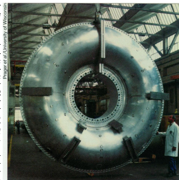
The thick metal walls of vacuum vessels like this one make it possible for scientists to study plasmas heated to solar temperatures in the laboratory.
