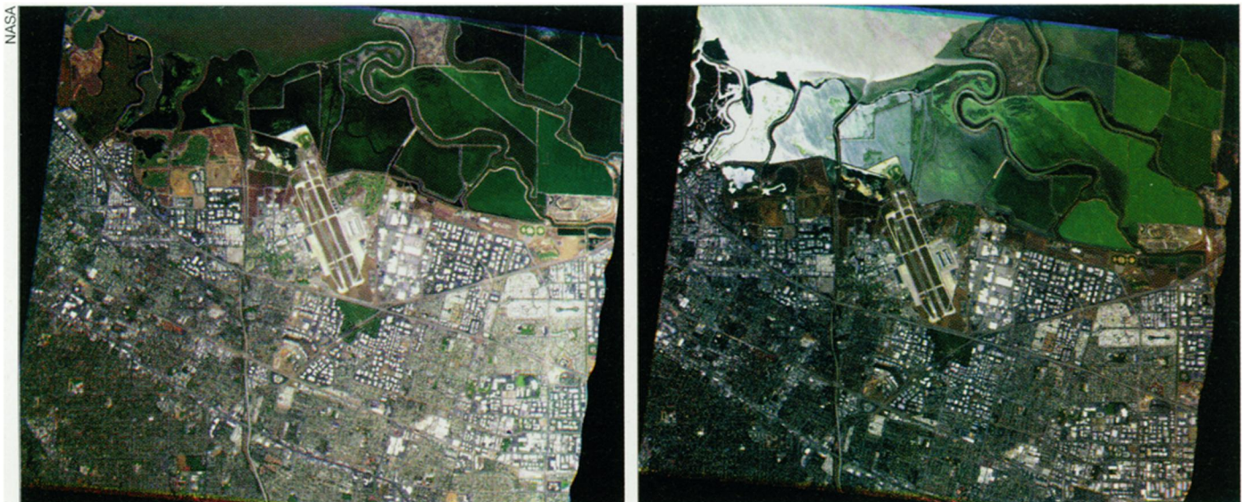
Room for two views. To get an example of how multiple images from the Terra satellite might appear, NASA put a stand-in for one of Terra’s instruments on a high-flying aircraft. From an altitude of 20 kilometers, cameras collected these images of San Francisco Bay and the cities of Mountain View and Sunnyvale. The only difference: One image is from a camera pointing forward on the plane, the other, a camera pointing rearward. The differing light angles yield distinct colorations.
