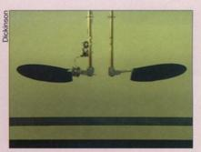
Measurements on these 25-centimeterlong Plexiglas wings, slowly flapping in mineral oil, probe equivalent aerodynamics of 1-millimeter-long fruit fly wings, which beat 200 times per second in air.
