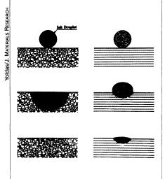
When an ink droplet soaks into a porous film (left), much of the dye is pulled below the surface, decreasing the intensity of the color. Another type of film (right) swells when it absorbs an ink droplet. When the water later evaporates, the color stays near the surface.
