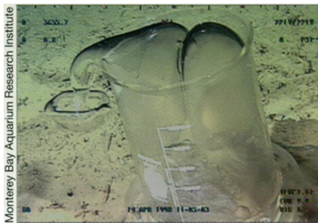
In the first deep-sea experiment of its kind, researchers pumped liquid carbon dioxide into a beaker 3.6 kilometers below the ocean surface. The carbon dioxide expanded and spilled out. A thin layer of icelike hydrate forms a coating around the carbon dioxide.
