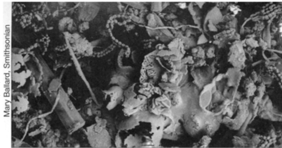
A sample of dust vacuumed from the Star-Spangled Banner includes clay particles, vegetable matter, synthetic fibers, and lint magnified 300-fold.
