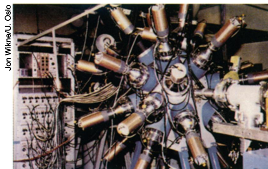
This instrument, called CACTUS, detects helium particles and gamma rays emerging from excited nuclei that undergo low-energy transitions.
