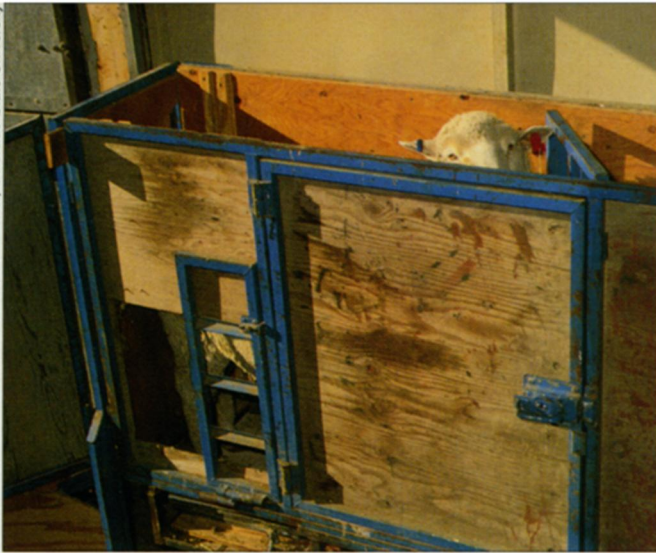
In a just-completed 2-year study, researchers put the hind legs of aging ewes—a model for osteoporosis in people—on this vibrating platform for a daily shake. The vibrated legs lost less bone than the animals' untreated forelegs. Depending on the frequency of the vibrations, some bones gained mass.
