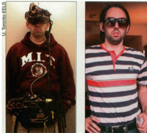
Shrinkage of computers, displays, and other gear has made "rigs" worn today by wearable computer pioneers smaller and more comfortable than earlier versions. The electronics that weighed down Steve Mann in the early 1990s (left) now fits into devices tucked discreetly into sunglasses, a one-hand keyboard in left hand, and hidden flaps in Mann's clothes (right).
