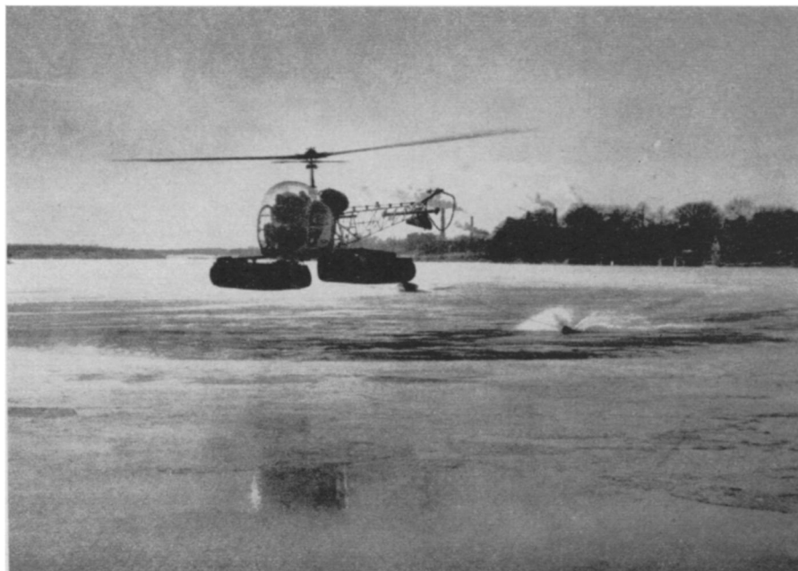
WILL SCAN ARCTIC OCEAN—The 47G-2A helicopter, made by Bell Helicopter Company, Fort Worth, Tex., demonstrates in the ice-coated water of St. Lawrence River how hydrographic sounding gear will be used for charting the ocean floor in arctic regions.
