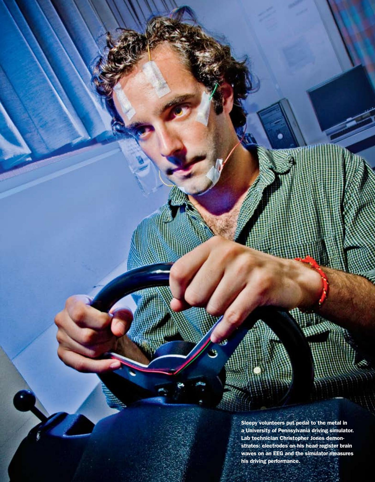
Sleepy volunteers put pedal to the metal in a University of Pennsylvania driving simulator. Lab technician Christopher Jones demonstrates: electrodes on his head register brain waves on an EEG and the simulator measures his driving performance.
