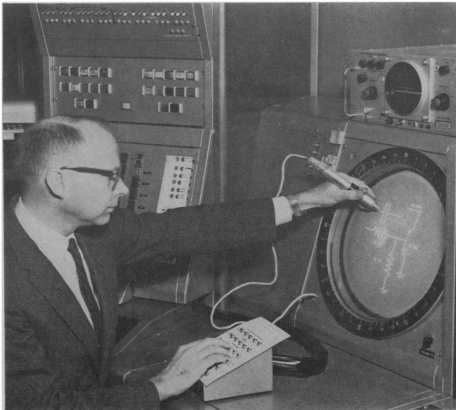
MAGIC—Paul Meissner, an engineer at the National Bureau of Standards, uses a light pen at MAGIC (Machine for Automatic Graphics Interface to a Computer) to connect an added symbol to a schematic drawing obtained from the machine's memory.
