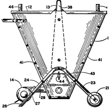
bottom feeds air through a perforated pipe to the stack. The sides of the burner are angled so that refuse to be burned won't pack up against the blower pipe and block the flow of air.
