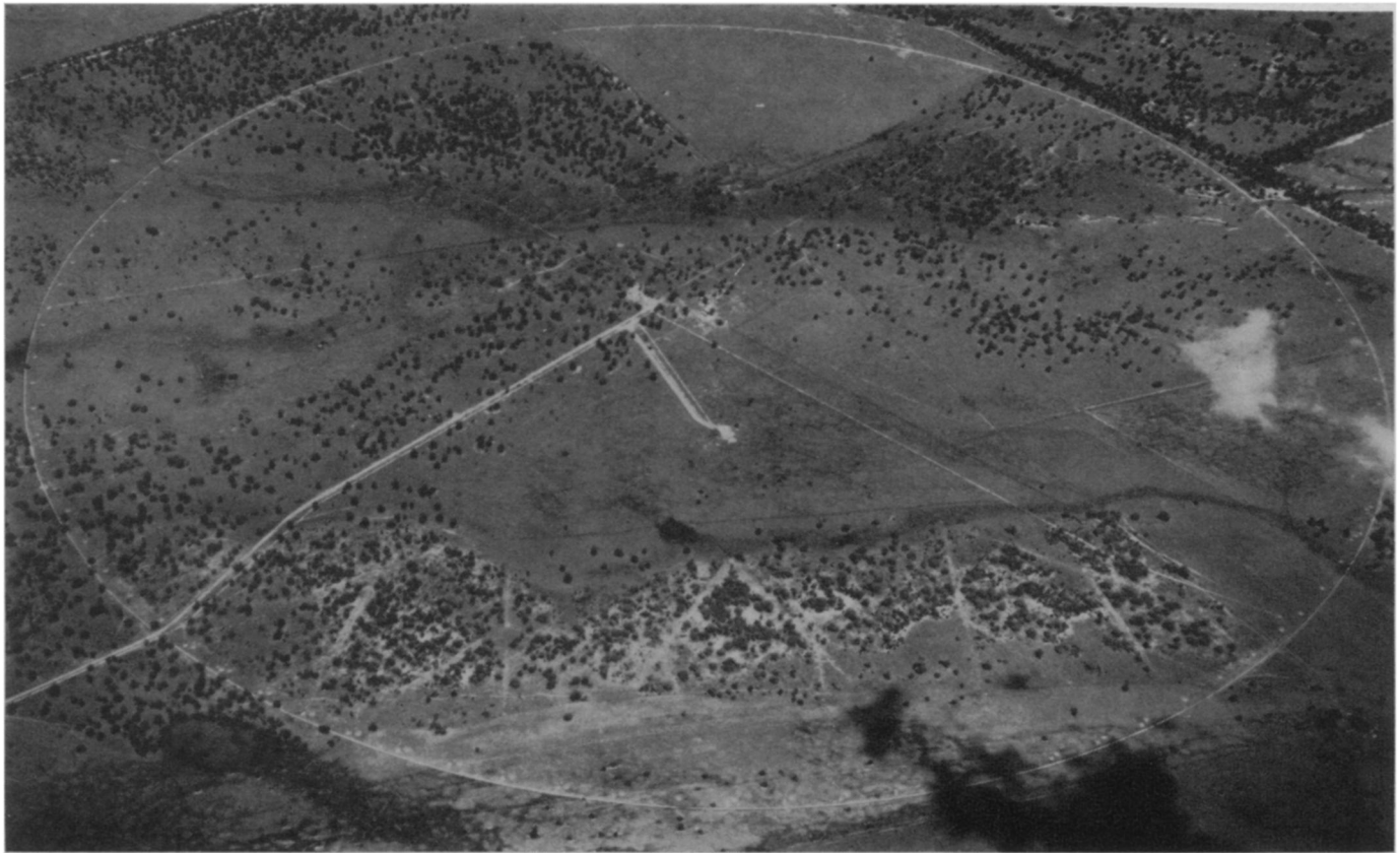
Culgoora, Australia, radioheliograph. The circle's 96 interconnected dishes observe the sun simultaneously.
