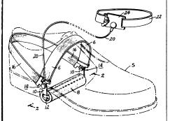
Co. of New York. A hollow tube of conducting material contains a metal rod that can be connected by wire to a clamp on the leg. When a charge builds up on the body, it can flow to the rod which is pressed against the cylinder when the wearer steps down.
