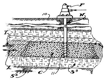
California, uses a second well in addition to the one through which the fresh water is being extracted. Fresh water is pumped down this second well both to maintain pressure in the aquifer and to keep a current flowing against the incoming salt water. This is obviously less than ideal, however, since the whole idea is conservation of limited fresh water.
