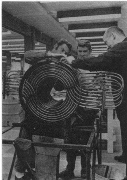
Setting up a modern boiler for testing.
