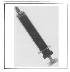
Gas syringes extract or inject gas samples from or into gas chromatographs, instruments that analyze the composition of gases. Like the familiar hypodermic, they have a plunger, which moves up and down in a glass tube. The interface between the surface of the plunger and the contents is a potential trouble spot because gas can leak out.
