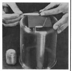
ous materials, it is useful for cementing conductors and terminals on electronic components. It is cured after application by baking at 400 to 500 degrees F.
