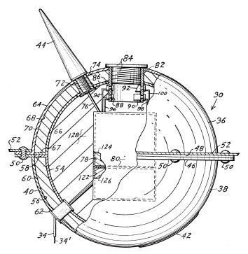
broken, or it can be turned on manually. Half a dozen layers of casing and insulation are intended to armor the transmitter against just about anything, possibly including even a direct hit.
