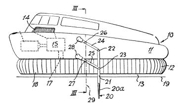
device's shallow draft, however, it still cancels a major advantage of most existing hovercraft, which are driven by propellers in the air: the ability to go on both land and water. Cockerell's invention is limited to non-amphibious hovercraft.
