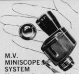
Monocular of outstanding design and performance. Fits in the palm of your hand. More powerful than most standard binoculars and field glasses. Standard objective 8x, 24mm., 8.2°. Extra objective: 6x, 18mm., superwide 11°! Prismatic, fully coated optics—crisp, brilliant and of complete planarity. Objectives may be used as 3x and 5x amplifier/loupes of unexcelled definition and clarity. 3½ ozs., 3½ inches. With zippered case and handstrap. \$16.95
