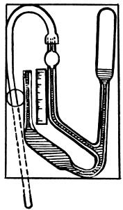
Construct low priced McLeod Gauge designed for student and amateur use. Includes pyrex gauge with case, plastic tubing, hardware and seal. Directions for calibration.
