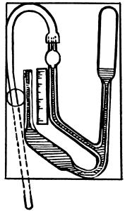
Construct low priced McLeod Gauge designed for student and amateur use. Includes pyrex gauge with case, plastic tubing, hardware and seal. Directions for calibration.
