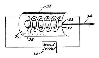
ruby crystal. This optical energy excites the ruby atoms to a higher energy state, from which the energy is reradiated almost entirely in one frequency band. The excited atoms are coupled to the atomic resonator and stimulated to emit their radiation together.
