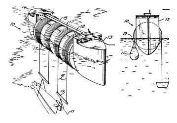
flooded; as this happens, the counterweight's torque is applied to the sunken object, lifting it. The maximum lift capacity of the rig is said to be much greater than conventional hoisting gear.
