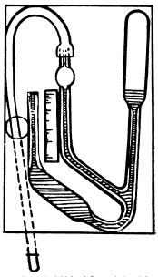
Construct low priced McLeod Gauge designed for student and amateur use. Includes pyrex gauge wit case, plastic tubing, hardware and seal. Direction for calibration.
