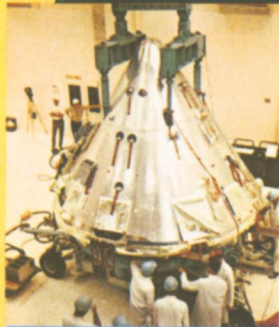
WITH A FINE-TOOTH COMB! Technicians carefully inspect Apollo command capsule before shipment.
