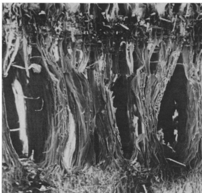
Electron micrograph of cross section of a cast fabric sample and a bolt of the material with its developers.
