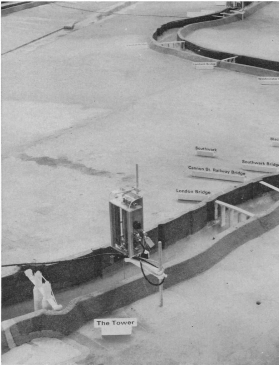
Scale model Thames simulates what happens when tide and North Sea combine.
