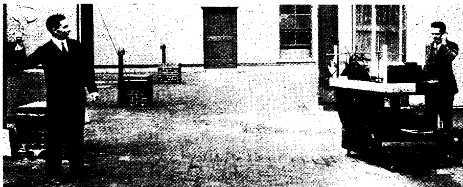
THE LATEST IN TELEVISION. The apparatus used in recent daylight television tests when full length figures of men playing tennis, or boxing, on the roof of the Bell Telephone Laboratories in New York, were seen by wire in a room several floors below. In actual use the transmitter, at the right, is covered so that it is lightproof. There can be seen the large scanning disc, which breaks up the image of the lens into small parts, like the dots of this half-tone picture when viewed with a magnifying glass.
