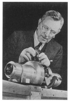
POWER BY RADIO Transmission of power by radio has been successfully accomplished with this tube in a demonstration by Westinghouse scientists. It is shown with I. M. Mouromtseff, one of the engineers who developed it.
