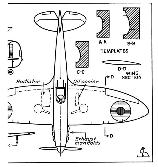
Ltd., Southampton, England. It is powered with one Rolls-Royce, 1,030 h. p. engine, which gives it a speed of 387 m. p. h.
