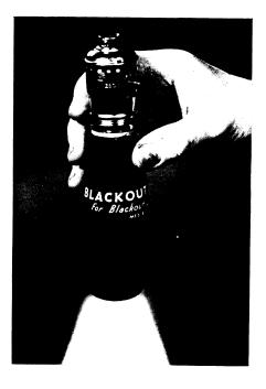
black silicate down to the extreme lighting end of the bulb insures that no trace of light escapes through the sides. The end of the bulb is a deep blue. The lamp consumes 25 watts and despite its silver lining is very inexpensive.
