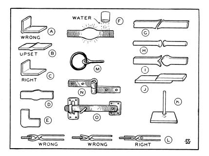
Diagram K illustrates the making of such things as metal stands, engine valves, etc. Note that the bottom of the rod is rounded. This fits into a slight depression in the plate. Both pieces must be heated to welding heat and then hammered together.
