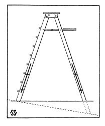
An extensible stepladder has lately been patented in which each of the four legs can be independently lengthened somewhat so that the ladder can be adapted to sloping or uneven ground and still maintain horizontal steps and a level top. The illustration shows how, if the ground slopes down, the back legs
