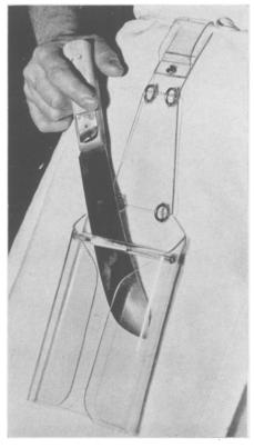
Transparent plastic replaces aluminum as a knife sheath for packing house workers. Aluminum had previously been used because of its lightness, but the plastic is still lighter and is not breakable. Moreover the sheaths are made from scrap remaining from construction of airplane turrets and win-
