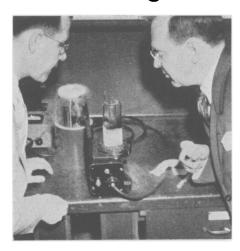
gummy at low temperatures. The vapor, which may be that of magnesium, chromium, gold, zinc, lead or, best of all, of barium, is sprayed on the bearing electrically and condenses to a thin soft lubricating film. In the picture scientists are watching a bearing lubricated with barium running at 314 degrees below zero Fahrenheit, in liquid air.
