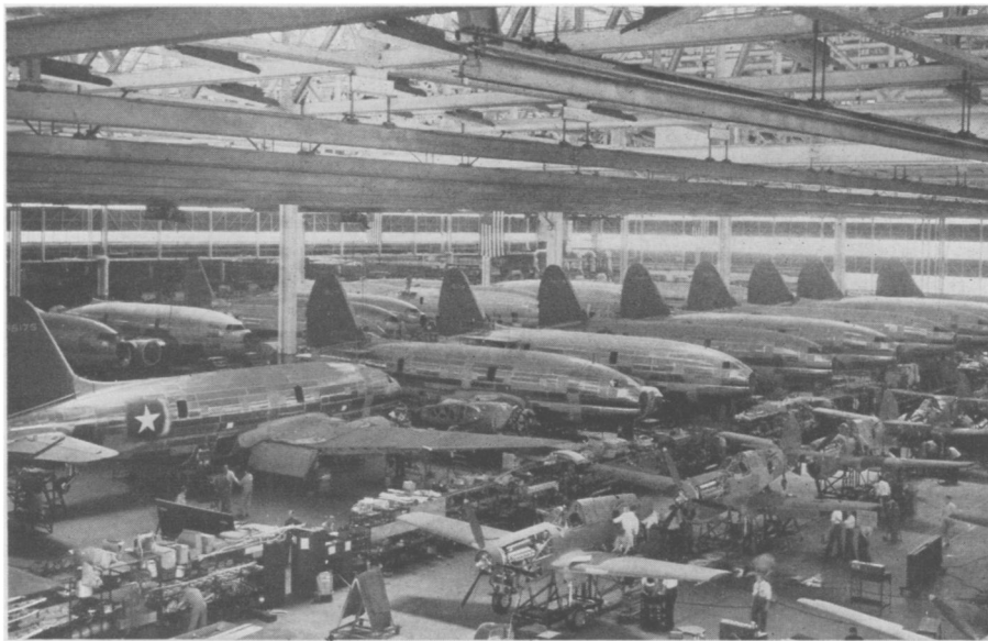
CARGO CARRIERS AND FIGHTER PLANES , turned out in increasing numbers at Curtiss-Wright, has won the company the joint Army-Navy "E" award for efficient production. Curtiss Commando military transports are shown in the background, while Kittyhawk and Warhawk fighters are seen being assembled in the foreground.
