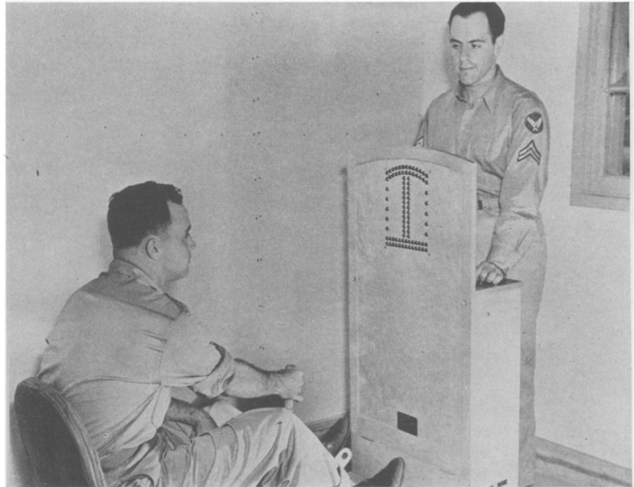
FORETASTE OF FLIGHT is given aviation cadets by new psychological tests being developed by Army scientists. This picture shows a cadet working joy stick and rudder bar in response to flashing light signals to determine his coordination of the movements of his hands and feet. Official photograph of U. S. Army Air Forces.
