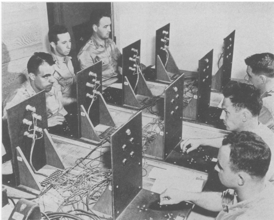
SPEED OF DECISION is tested when the cadet must operate the correct control in response to flashing light combinations as shown in this official photograph from the U. S. Army Air Forces.
