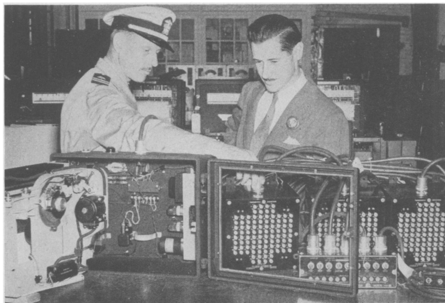
FLIGHT RECORDER —Lieut. William C. Clay, Navy flight test officer inspects the ingenious electronic robot that obtains data in the flight testing of airplanes. The device was developed by the Brown Instrument Company.
