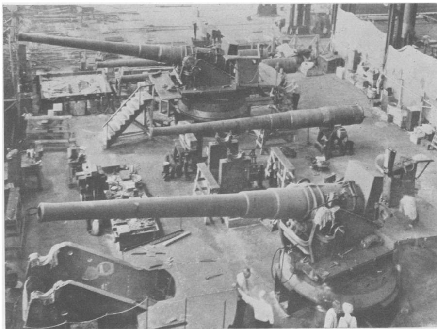
COAST ARTILLERY —Gun mounts in the shops of the Baldwin Locomotive Works. This famous builder of locomotives is now at work on several types of war material. The mounts shown weigh 250,000 pounds each and are built from steel castings produced in Baldwin foundries.
