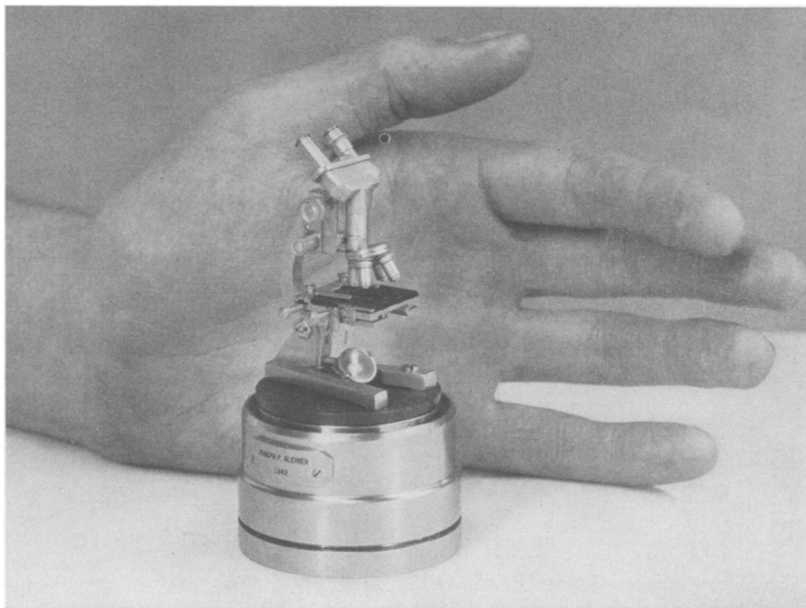
MICROSCOPIC MICROSCOPE —Working with watchmaker's lathe, taps, and dies, Joseph P. Kleiber, Bausch and Lomb microscope worker made this tiny model of a standard instrument. It is only two and three-quarters inches high and is a binocular type microscope with revolving eyepiece carrying three objectives.
