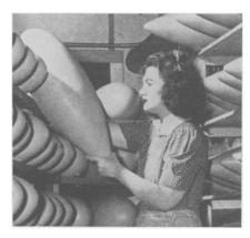
ANTENNAE HOUSINGS that look like bombs were part of the equipment on the B-25 bombers that raided Tokyo. They are tear-shaped structures made of plastic. When news of their part in Gen. Doolittle's flight reached the factory of these devices, the employees tripled production overnight.
