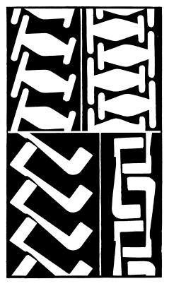
SAVING—The layouts shown here show how precious metal is being saved in cutting pieces for war production. At the left is the way the patterns have been laid down when metal was more plentiful. At the right are economy layouts worked out by a General Electric Company expert.
