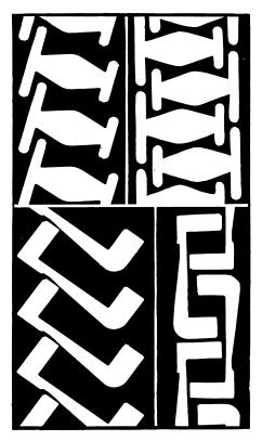
SAVING—The layouts shown here show how precious metal is being saved in cutting pieces for war production. At the left is the way the patterns have been laid down when metal was more plentiful. At the right are economy layouts worked out by a General Electric Company expert.
