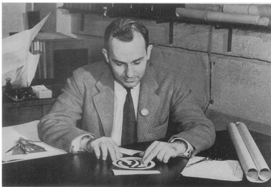
PLANNING —Working out a war-essential sort of jig-saw puzzle, J. C. Smith, General Electric Company planner, arranges a layout with paper pieces to insure minimum waste when the patterns are later cut from steel.
