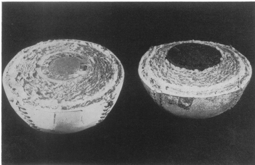
WAR BASEBALL —At the right is the new baseball made with a rubber-cushioned center borrowed from golf balls. It is compared with the old official cork-centered ball now out for the duration. The photograph is an official one of the Office of War Information.
