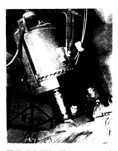
WAR X-RAYS—This 1,000,000-volt X-ray unit built by General Electric is being used to check welded seams in an Army tank. Energy is produced equivalent to \$90,000,000 worth of radium. Thicknesses of metal can be inspected in minutes which formerly required hours.
