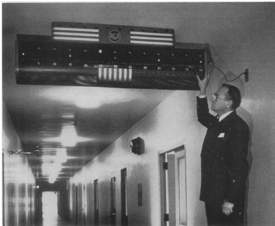
ELECTRONIC CLOCK —The more than 170 electronic tubes in this modern clock count the 60-cycle pulsations of electric current and show the seconds, minutes and hours by lights. The seconds are ticked off on the line shown from one to 60; other lights indicate the hours and minutes. The clock has no moving parts—no motor, wheels, main spring or hands. With the clock is shown Dr. V. K. Zworykin, associate director of RCA laboratories, who with his staff developed it.
