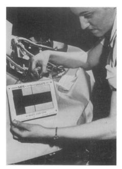
dow, bound together in a cardboard frame as shown in the photograph. This is placed inside the protective covering. Moisture causes the crystals to turn pink.
